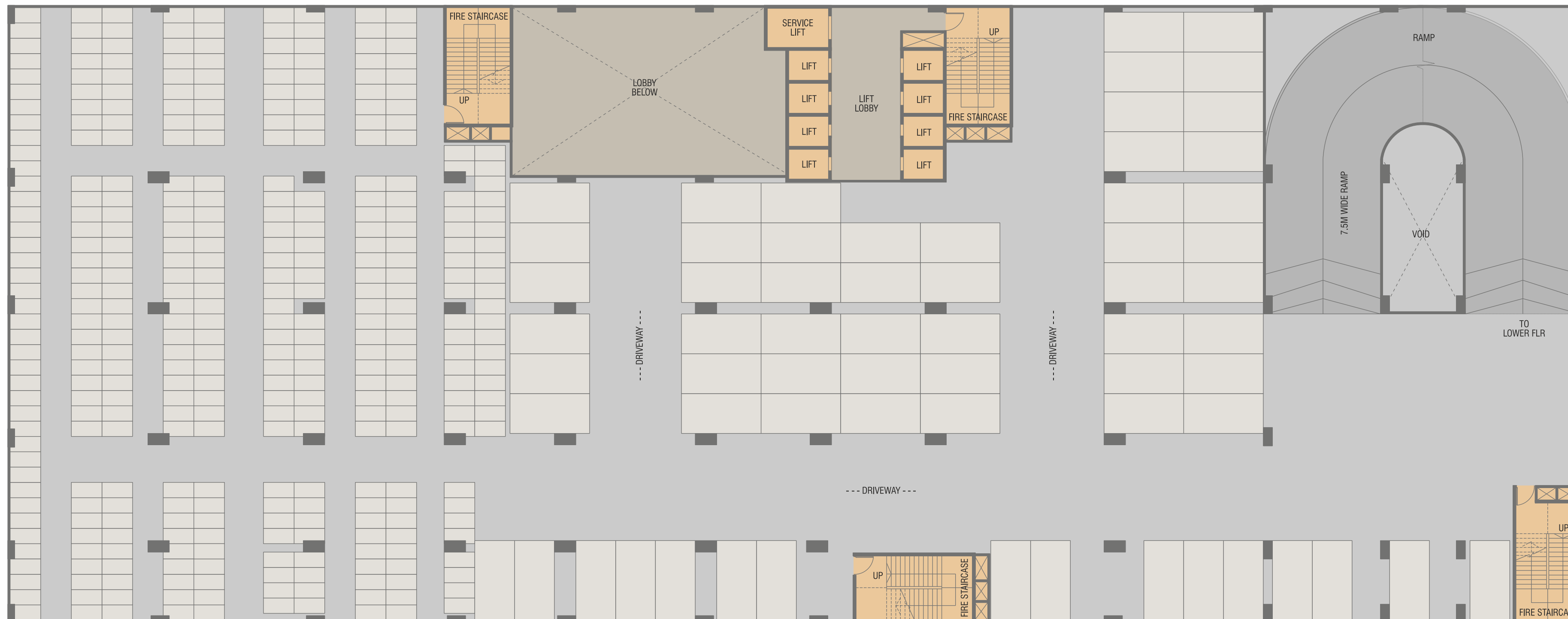
PARKING 1 FLOOR PLAN FOUR WHEELERS (MECH. PUZZLE+STACK) & TWO WHEELERS
