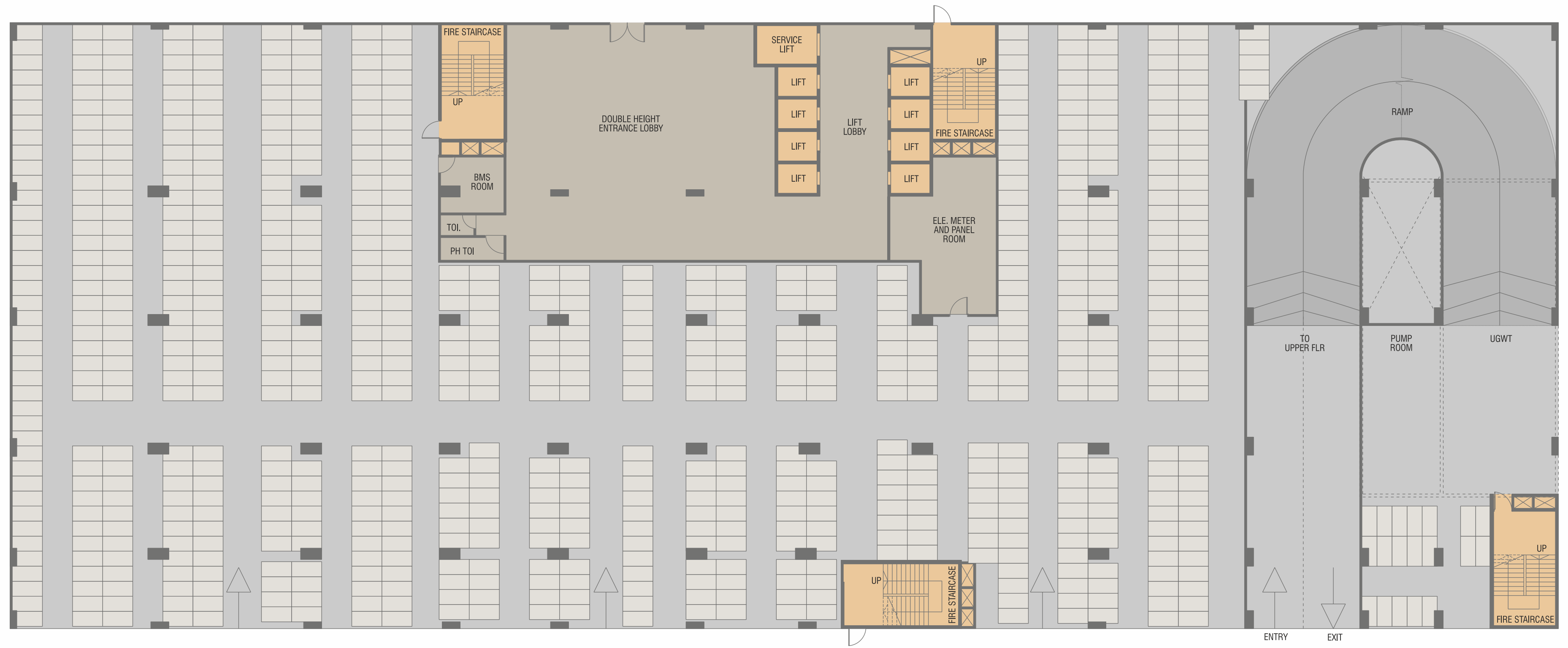
GROUND FLOOR PLAN TWO WHEELERS PARKING
